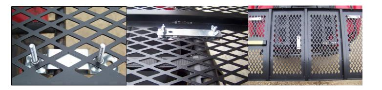
WARNING: The Harty Hauler is intended to be installed on tubular ATV racks only and must lay flat.
