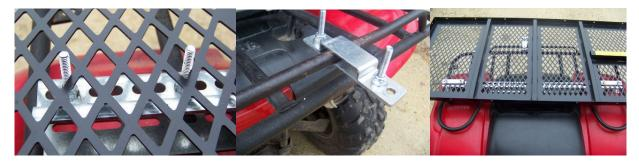
WARNING: The Harty Hauler is intended to be installed on tubular ATV racks only and must lay flat.
